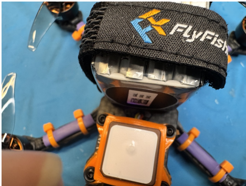
Actual BZ-181 M10 installation: give the antenna a clear view of the sky.
