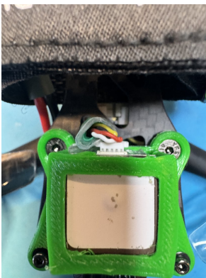
GPS detail from the catalog. Keep its mount secure and give it a clear view of the sky for outdoor acquisition.
