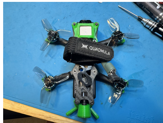
Top view: keep the strap and both battery leads clear of the propellers.
