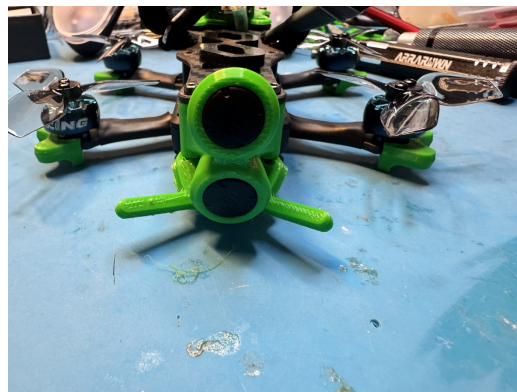
Rear view: inspect the custom antenna mounts and keep antenna elements clear of damage and rotating parts.
