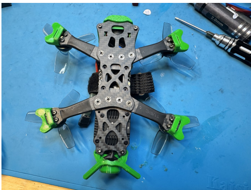
Underside view: inspect the carbon, fasteners and motor-wire routing before powering the aircraft.
