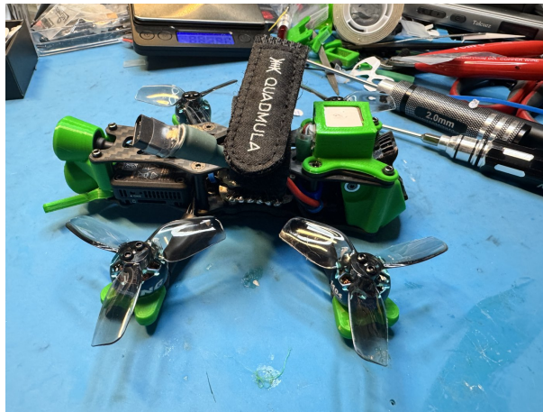
Assembled aircraft: confirm prop, strap and wiring clearance each time you install a flight battery.
